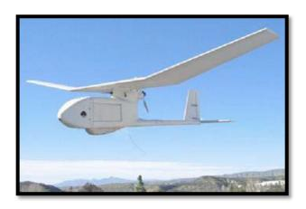
location data. The Raven is battery-powered and can stay airborne for up to 90 minutes at speeds up to 50 mph. <sup>17</sup> It can operate day or night.
